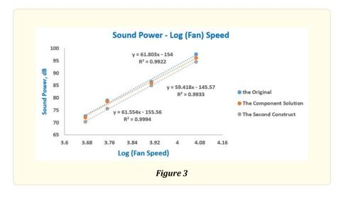
It should be reminded that Figure 3 shows the reduction of the noise level (please note that x is log RPM and y is the Sound Power). One may ask the question why we stopped at the second construct. To answer, we should remind that there is a constraint in the system which is the air flow (See Appendix B).
