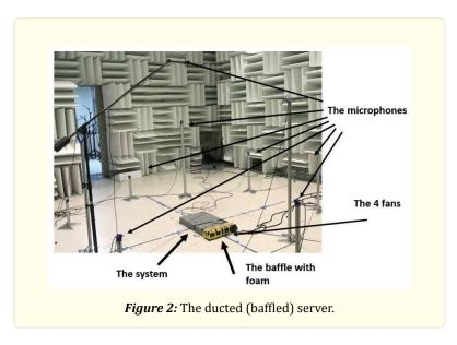
In reaching this design, the first construct was to add the baffle. Then the second Construct was creating a partition for each fan (see figure 2).
